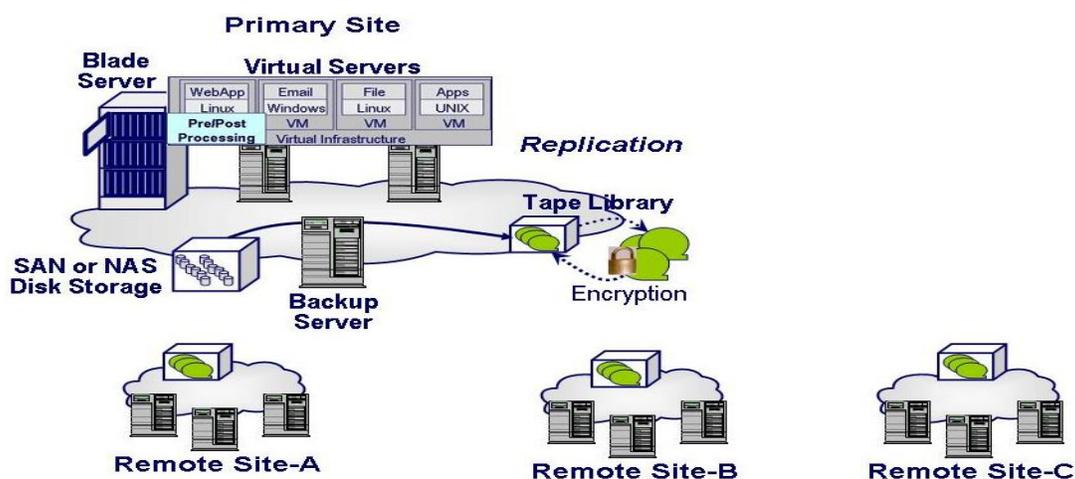
Figure-1: Providing High Availability and Protecting Local and Remote Virtual and Physical Servers
